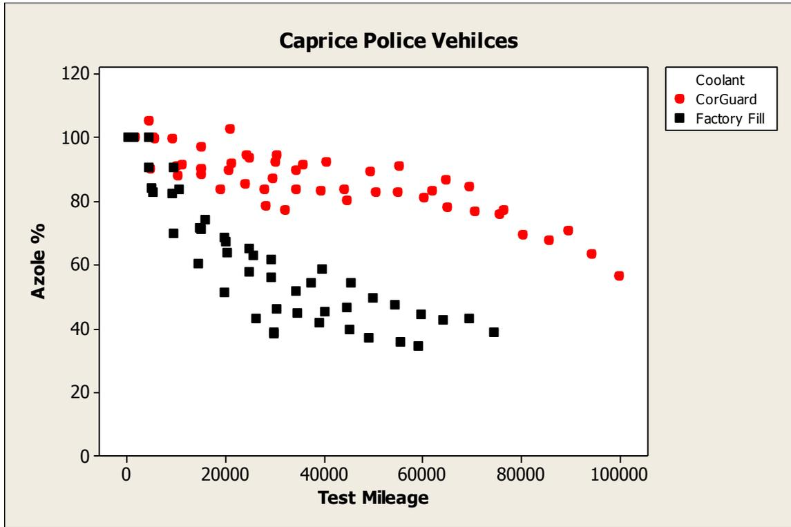
Figure 12. Total Azole, % as a function test mileage – Prestone Cor-Guard and GM Factory Fill coolants.
