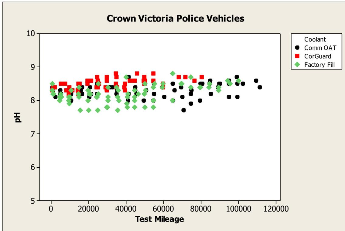
Figure 2. Test Coolant pH vs. test mileage for – Commercial OAT, Prestone Cor-Guard and Ford Factory Fill coolants.
