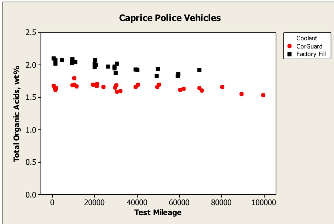
Figure 11. Total Organic Acid level as a function test mileage – Prestone Cor-Guard and GM Factory Fill coolants.
