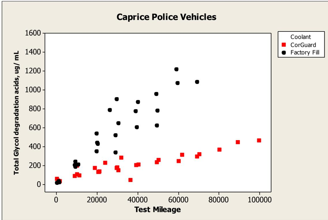
Figure 9. Total glycol degradation acid concentration as a function test mileage –Prestone Cor-Guard and GM Factory Fill coolants.
