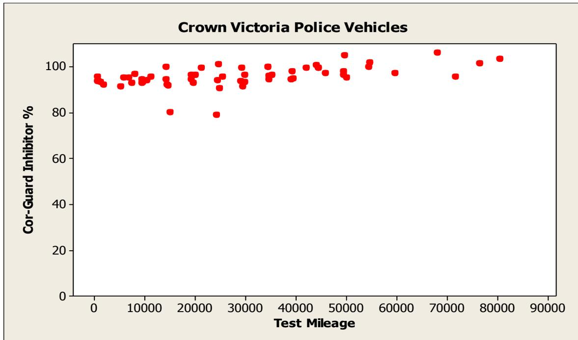
Figure 5. A key Cor-Guard Inhibitor % levels vs. test mileage for – Prestone Cor-Guard coolant.
