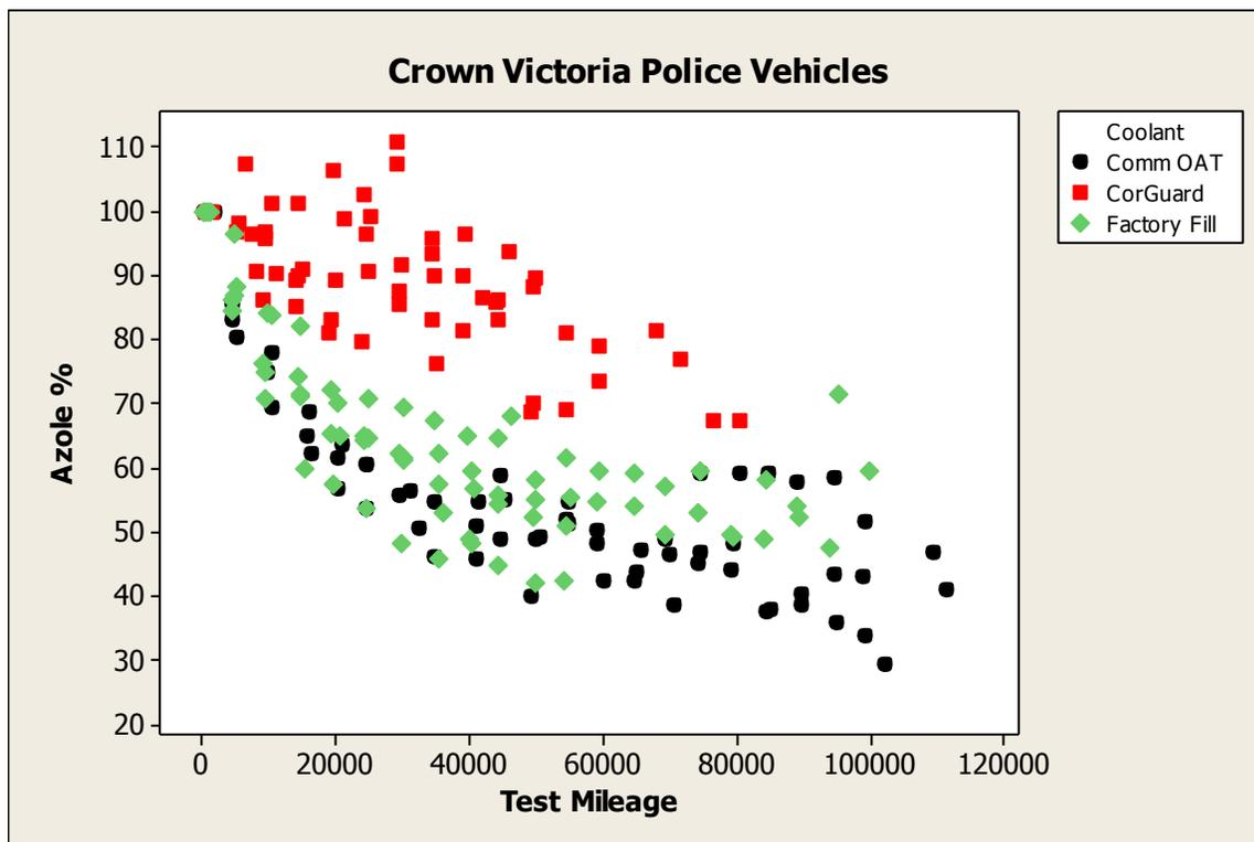
Figure 4. Azole % levels vs. test mileage for – Commercial OAT, Prestone Cor-Guard and Ford Factory Fill coolants.
