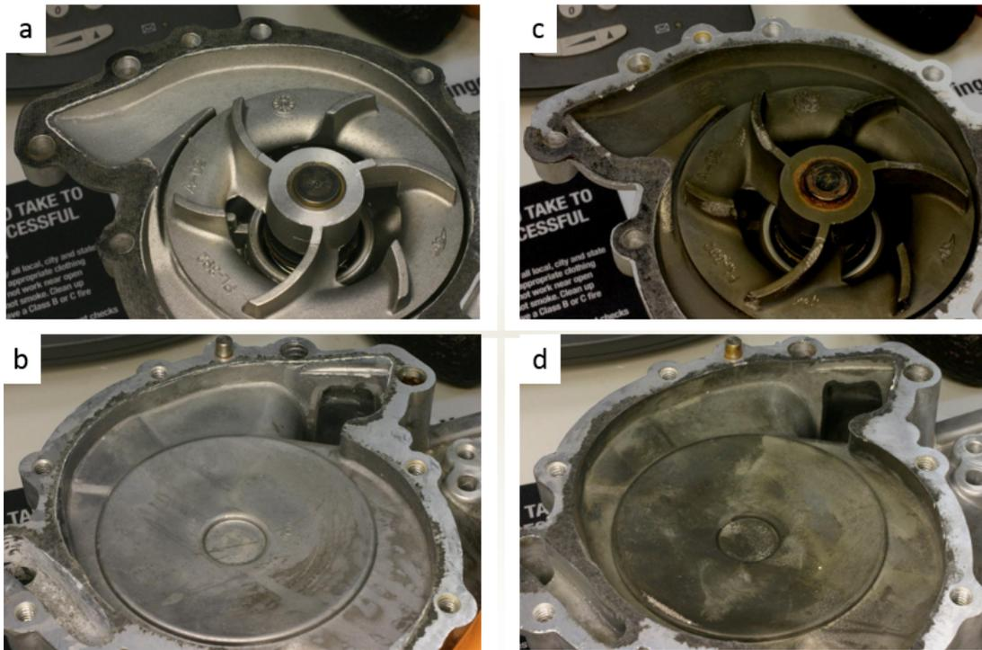
Figure 8. ASTM D2809 pump test result in stainless steel unit by internal laboratory a) pump and b) pump cover for Prestone Cor-Guard; c) pump d) pump cover for the Commercial Extended Life OAT coolant
