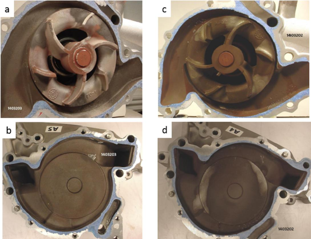
Figure 7. ASTM D2809 pump test result by outside independent laboratory a) pump and b) pump cover for Prestone Cor-Guard; c) pump d) pump cover for the Commercial Extended Life OAT coolant.
