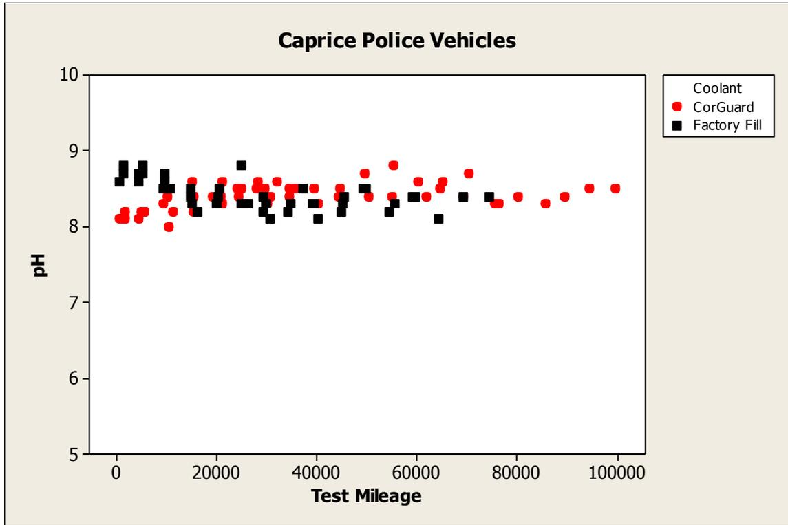
Figure 10. pH level as a function test mileage –Prestone Cor-Guard and GM Factory Fill coolants.
