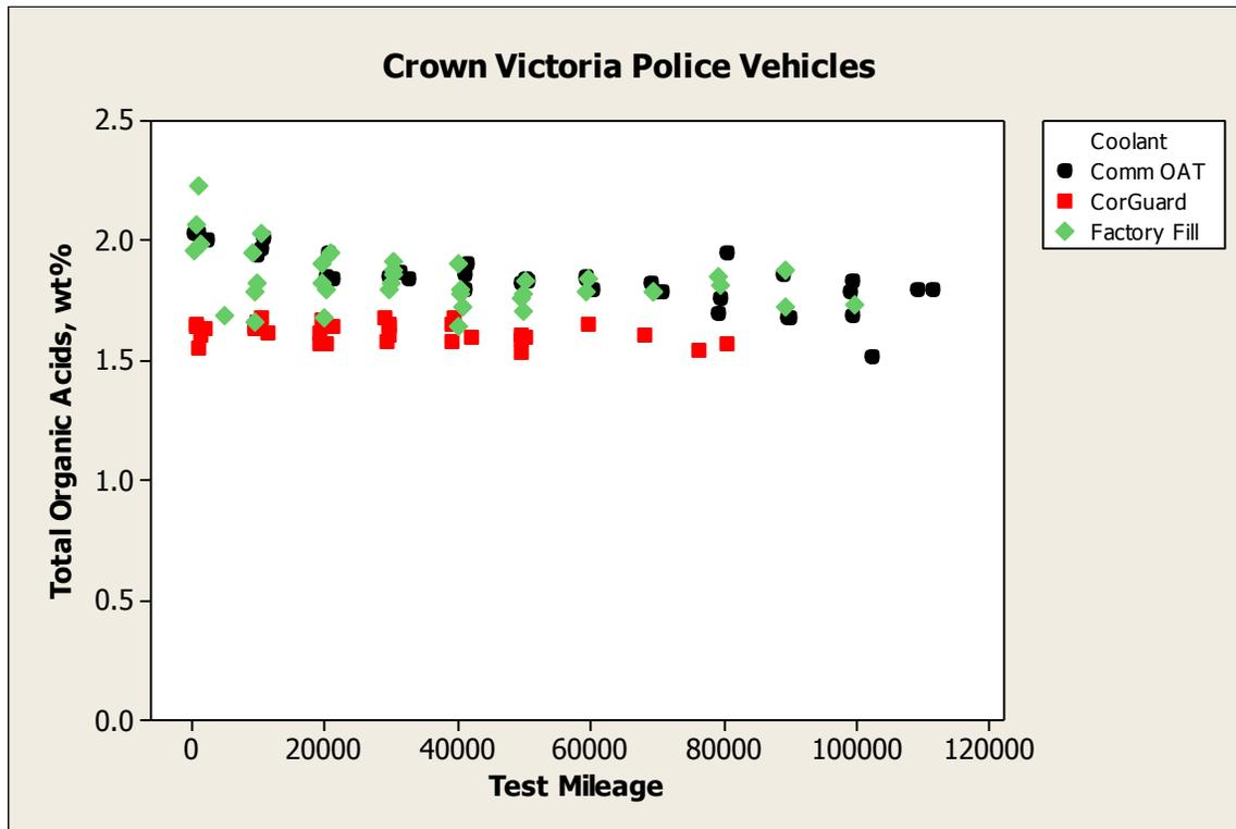
Figure 3. Total Organic Acid levels vs. test mileage for – Commercial OAT, Prestone Cor-Guard and Ford Factory Fill coolants.
