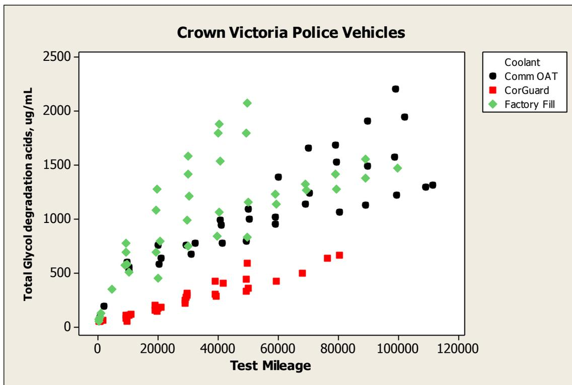
Figure 1. Total glycol degradation acid concentration as a function test mileage – Commercial OAT, Prestone Cor-Guard and Ford Factory Fill coolants.
