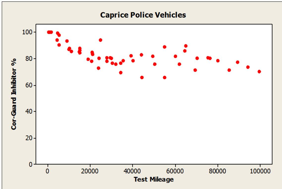
Figure 13. A key Cor-Guard Inhibitor % levels vs. test mileage for – Prestone Cor-Guard coolant.
